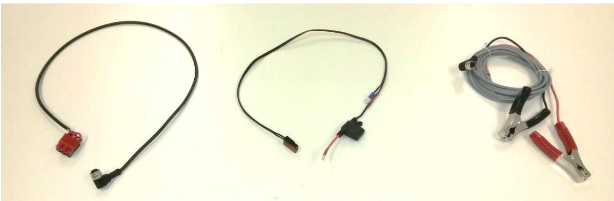
Power Supply Cable 12V with connector
